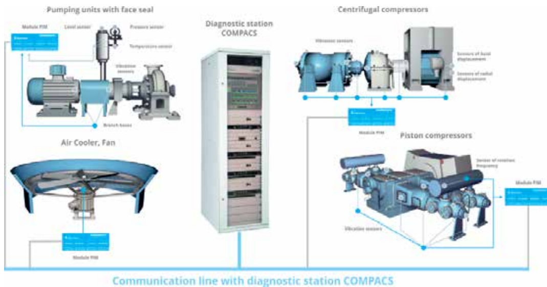
Figure 2. The COMPACS system monitors any machines of refinery Units
