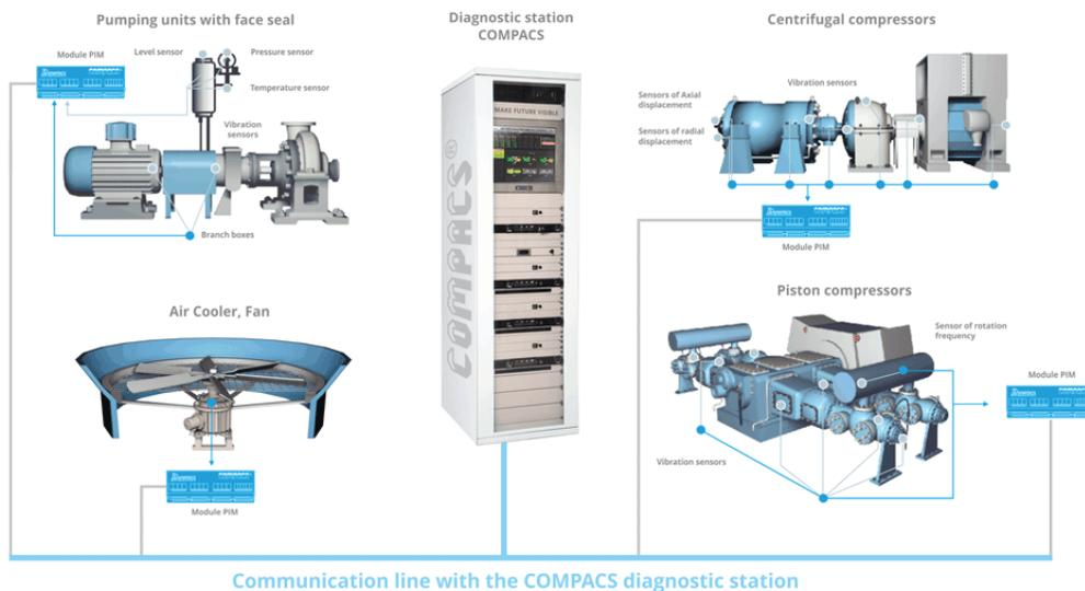
Figure 2. The COMPACS System monitors any machines of refinery Units
